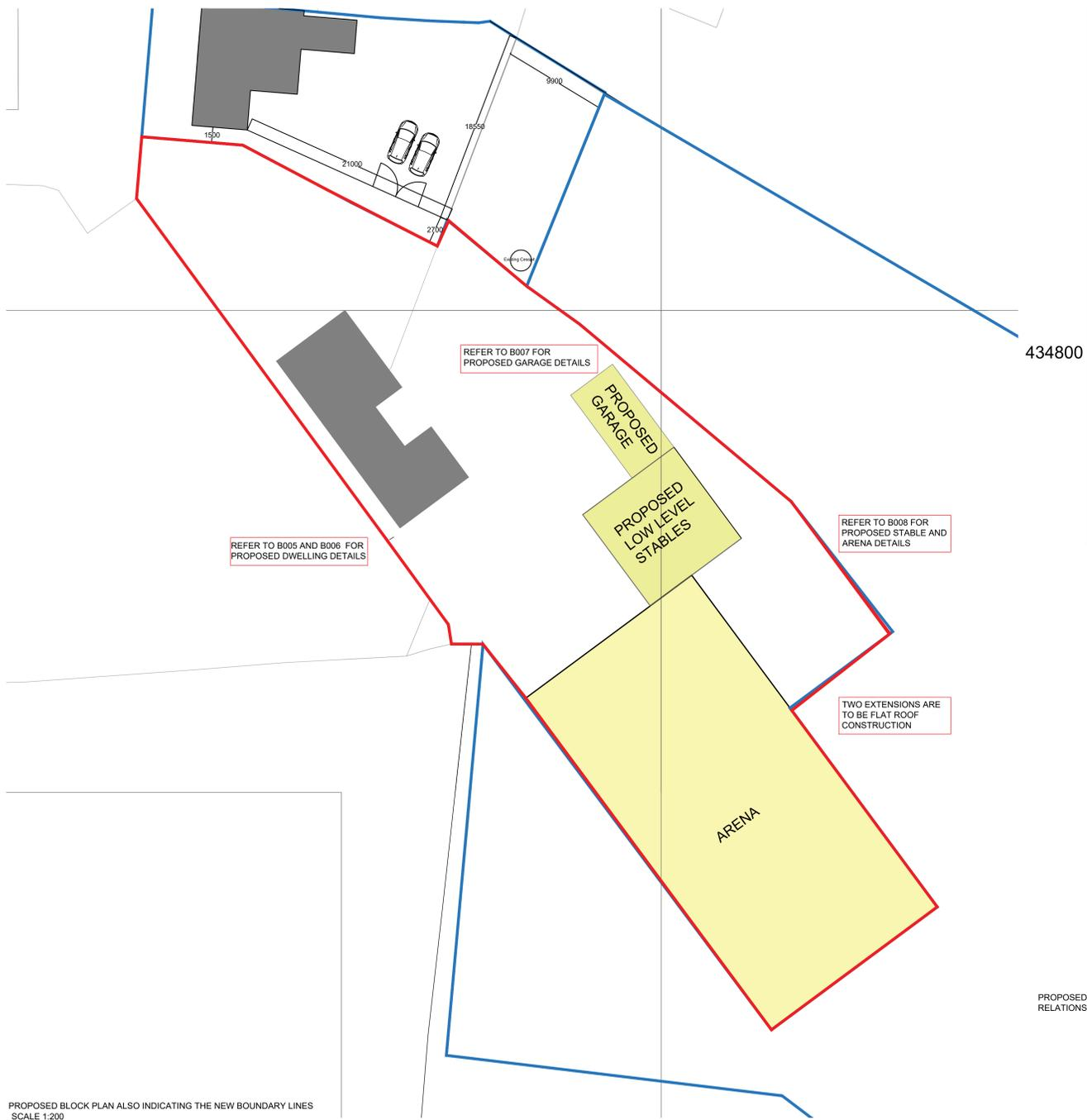
PROPOSED BLOCK PLAN ALSO INDICATING THE NEW BOUNDARY LINES
